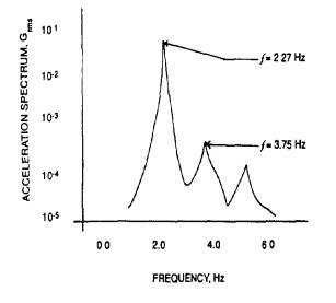
Fig. 4. Typical spectral response (floor excited by dancing).
