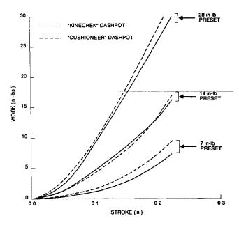
Fig. 8. Viscous dashpot work per stroke at various energy absorption settings. ("Kinechek" and "Cushioneer" refer to the manufacturer's
