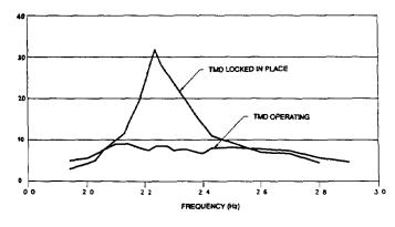
Fig. 11. Peak RMS floor response at tip of floor, subject to sinusoidal forcing function. Test of actual floor system with fieldtuned TMD (Crystal Quadrant).
