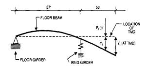
Fig. 5. Floor deflection in first mode shape (Section 1 in Fig. 2).
