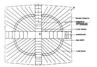
Fig. 2. Ballroom (6th floor) plan.
