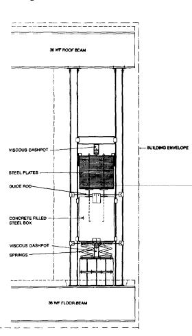
Fig. 10. TMD elevation.
