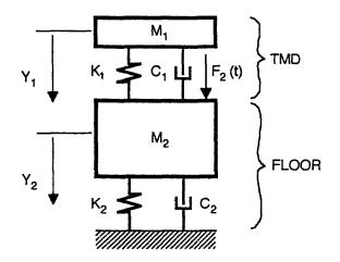
Fig. 7. 2 DOF floor-TMD model.
