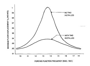
Fig. 9. Maximum, steady-state floor amplitudes at tip of floor, as predicted by Eq. 14. (TMD parameters correspond to "initial construction values" in Table 3.)
