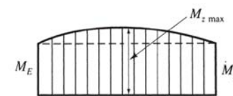
(c) Equivalent uniform moment with maximum magnified moment at midspan
