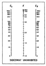
AISC specifies G = 10 for a pinned support and G = 1.0 for a fixed support.
